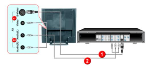
1. Input devices such as DVDs, VCRs or Camcorders are connected to the Video or S-Video terminal of the monitor using the RCA or S-VHS cable.
